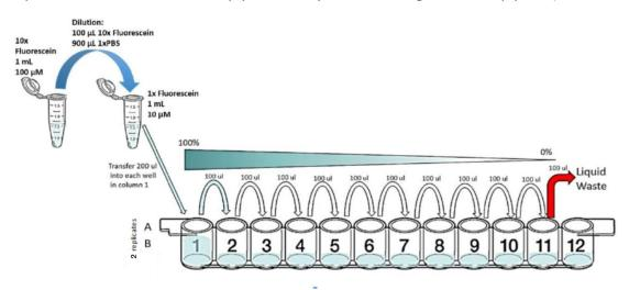
25. Discard 100.0uL from wells A11:H11 of calibration plate. This step ensures that all wells contain the same volume (100uL).
